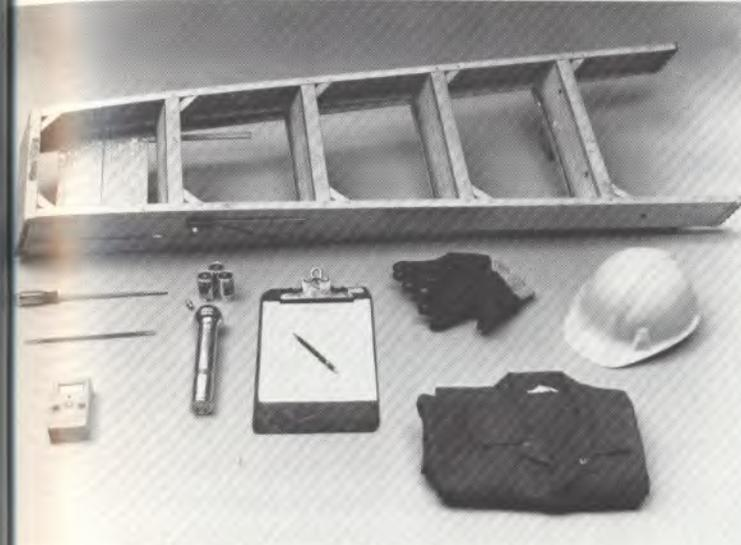
Figure 56. Inspection equipment: stepladder, screwdriver, hacksaw blade, moisture meter, flashlight with spare batteries and bulb, clipboard, inspection form, pen, gloves, bump helmet, and coveralls
