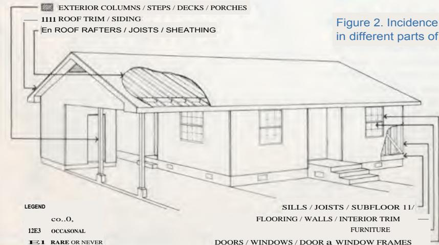
Figure 2. Incidence of damage in different parts of the house
