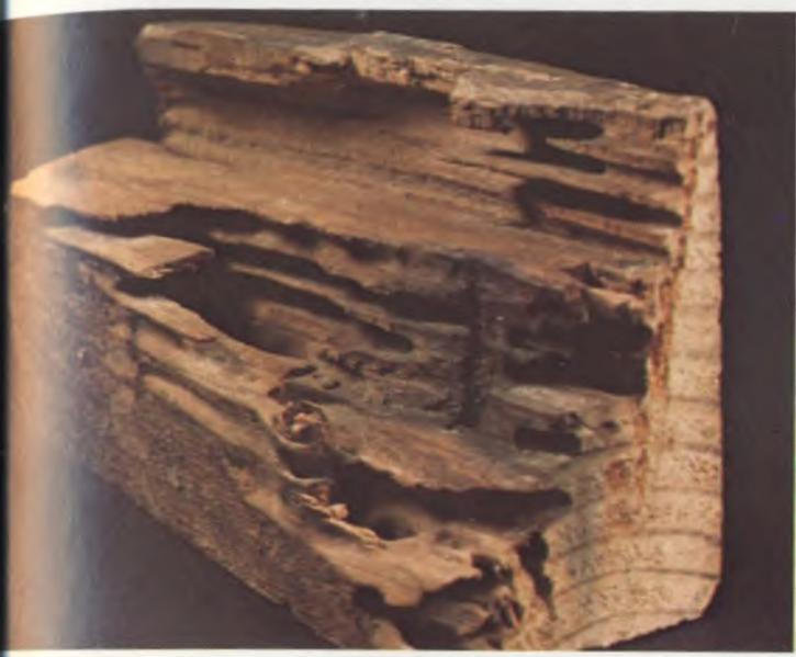
Figure 33B. Carpenter ant damage showing clean galleries with a smooth surface, the preferential attack the softer springwood, and some brown rot on end grain
