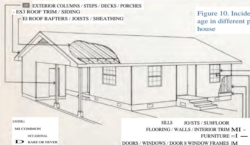
Figure 10. Incidence of damage in different parts of the house
