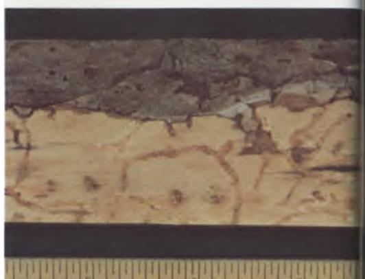
Figure 52. Bark beetle damage at bark/wood interface
