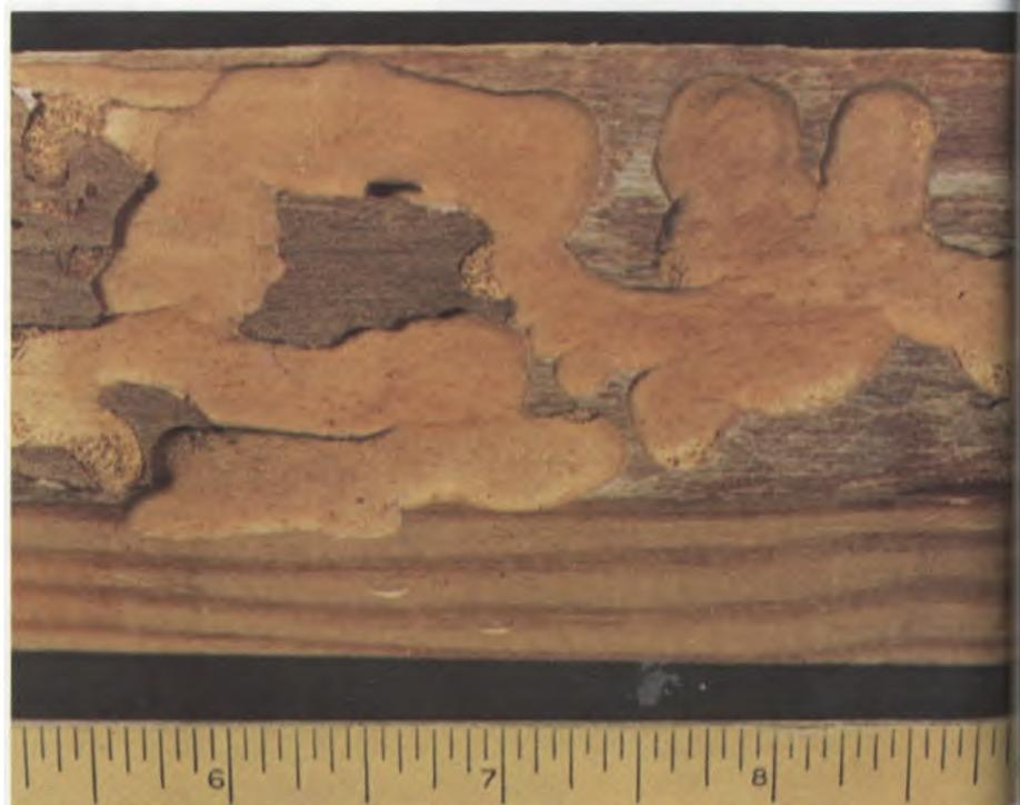
Figure 55. Flat-headed borer damage
