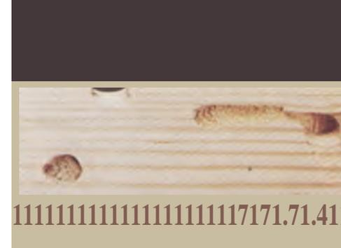
Figure 53. Horntail damage with characteristic circular galleries and tightly packed frass. Note slight stain around gallery in lower left corner.
