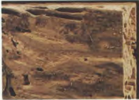
Figure 30A. Dampwood termite damage in one inch-thick board, showing some fecal pellets, the velvety appearance of the surface of the galleries, and the preferential attack of the softer springwood
