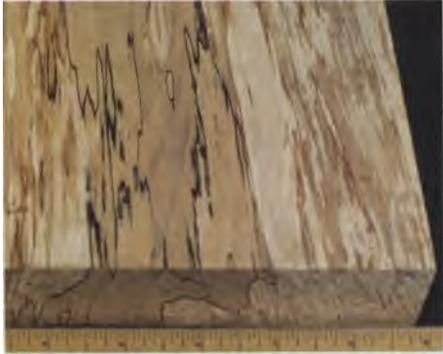
Figure 7. White rot, with black zone lines sometimes found in the early stages of decay
