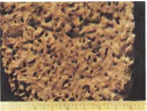
Figure 22. Carton produced between studs by Formosan subterranean termites
