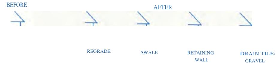
Drain rain water away from the house with gutters, downspouts and splashblocks: by regrading; or by attaching drain tile to downspouts to deposit the water in a storm sewer, dry well, or other location where it will not run under a house.
