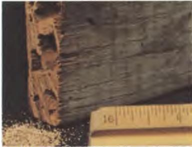
Figure 26. Drywood termite damage showing pellets, large chambers of galleries in the interior of wood, and small "kick-holes" on the surface
