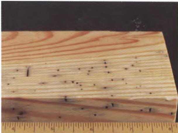
Figure 51. Ambrosia beetle damage with characteristic empty pin holes surrounded by darkly stained wood
