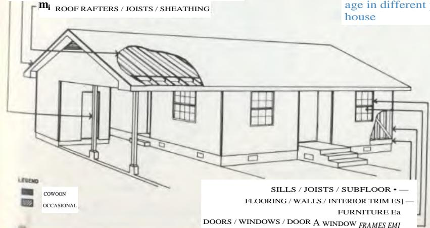
Figure 38. Incidence of damage in different parts of the house
