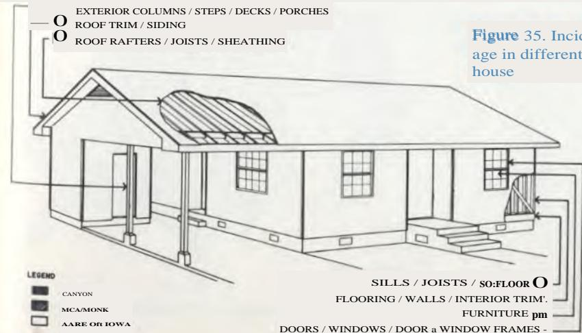
Figure 35. Incidence of damage in different parts of the house
