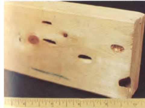
figure 54. Round-headed borer damage
