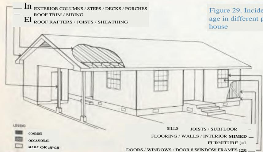
Figure 29. Incidence of damage in different parts of the house
