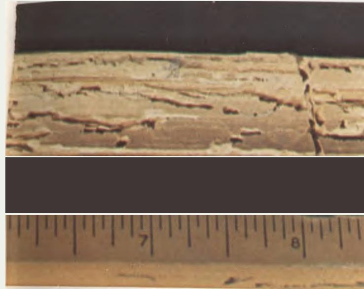
Figure 43. Bostrichid powderpost beetle damage in bamboo with exit holes on surface and some powder-filled galleries in the interior.
