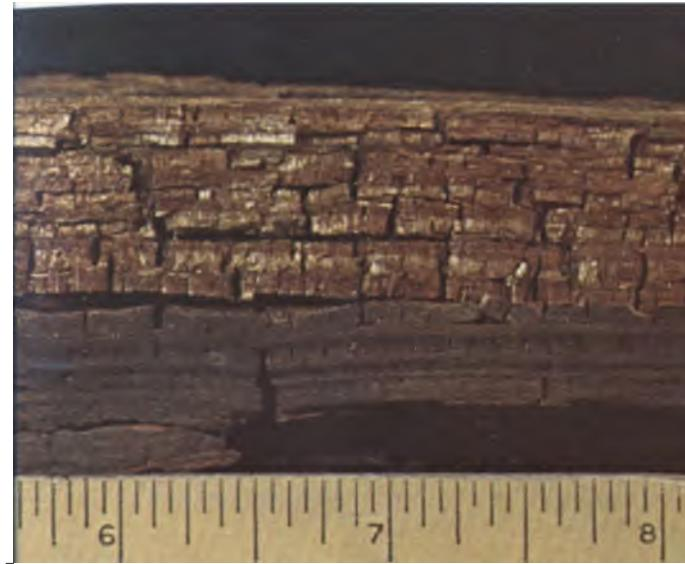
Figure 8. Brown rot, with characteristic cracks across grain
