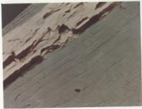
Figure 46. Old house borer damage with oval exit hole and powder-filled galleries in interior of wood
